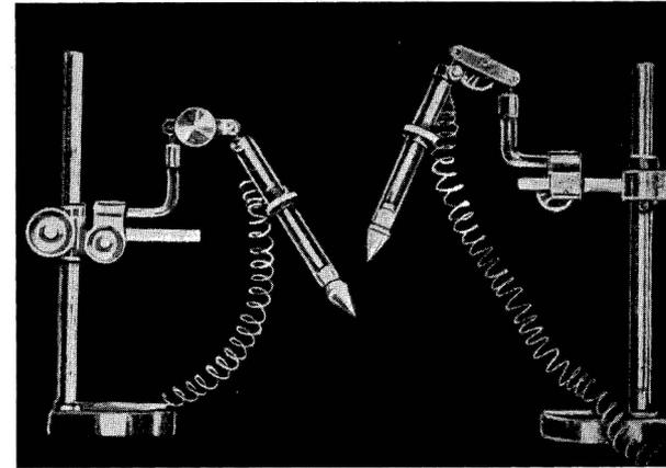
THE ELECTRODES USED BY BECK FOR RECORDING ELECTRICAL POTENTIALS FROM THE BRAIN
